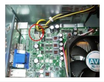
**5.4** ATX power cable insert and the cable need to rotate 3 times.
